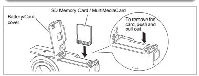
This camera uses an SD Memory Card and MultiMediaCard. Captured images are recorded on the SD Memory Card / MultiMediaCard if a card is inserted (in icon on the LCD monitor), or in the Built-in memory if no card is inserted (in icon on the LCD monitor). Make sure that the camera is turned off before inserting or removing the SD Memory Card / MultiMediaCard.
